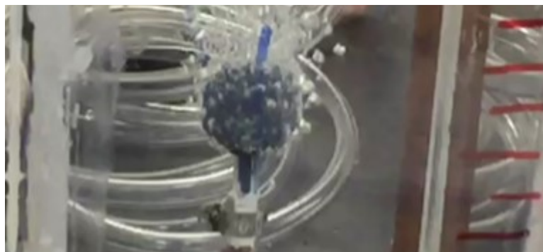
Figure 2.3: Pawfly air stone installed in the tank
